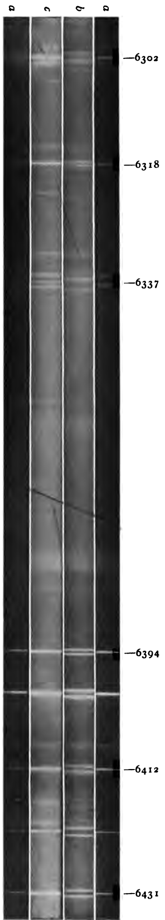
EFFECT OF MAGNETIC FIELD UPON THE SPARK SPECTRUM OF IRON. a. Spark without field. b. n -Components. c. p -Components.
